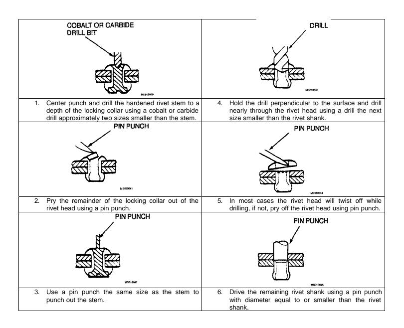
Figure No. 1: Rivet Removal
